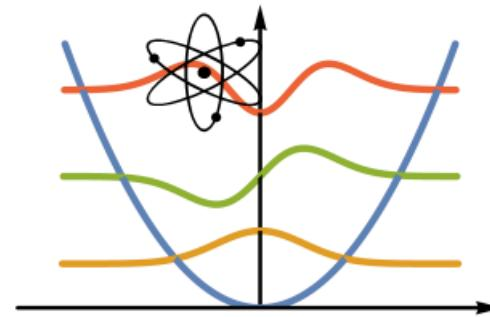
Typical trap frequencies:  $\sim 100$  kHz
