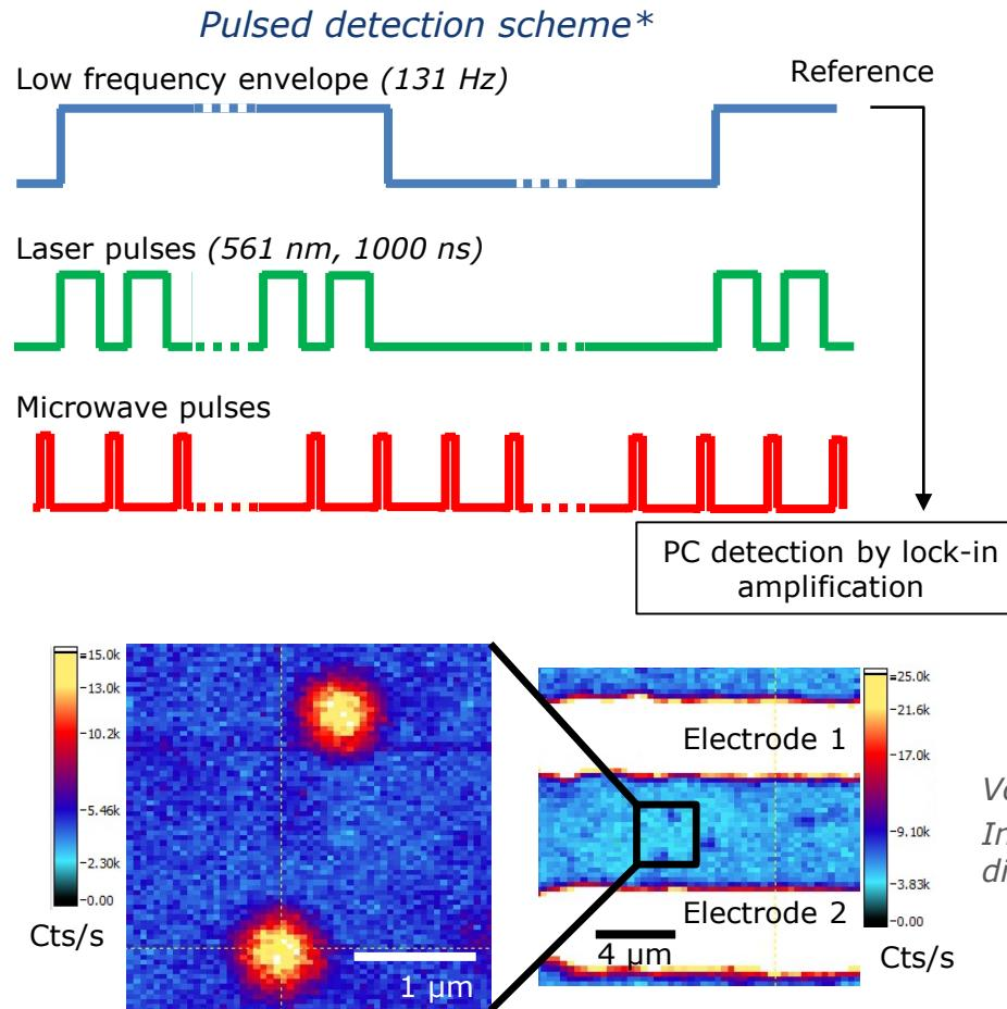
Photoelectric detection of Rabi oscillations on a single NV<sup>-</sup> centre
