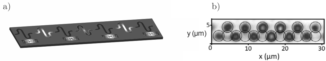
FIG. 1: Scheme of a density-wave of photons in a frustrated circuit QED lattice of alternating resonators, with qubits coupling to photons in every other resonator (a). Far field image of a polariton condensate in a lattice of micro-pillar cavities (b). The empty pillars are a signature of interference and geometric frustration.
