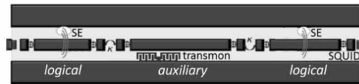
FIG. 1: Schematic representation of an elementary unit of our scalable setup to perform digital quantum simulation: logical resonators include ensembles of s = 1 spins placed at the magnetic field antinode of the respective superconducting resonator, where one of the spin transitions is in the strong coupling regime with the cavity mode; the auxiliary resonator contains a transmon coupled to the cavity mode electric field. The frequencies of individual resonators can be tuned by using SQUID devices.
